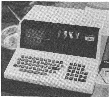
The Casio FX-9000P has removable memory units with on-board battery power.
