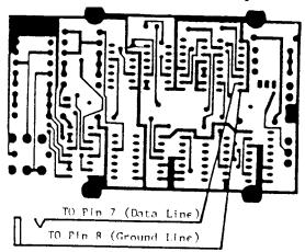
STEP 5: Using 2 color stranded wire, twist two pieces together to form a twisted pair. Referring to the above PC board diagram, connect one end of one wire to the ground side of the jack and the other end (same wire) to pin 8 of IC5(MC14503B). Connect one end of the unused different colored wire to the high side of the jack and the other end to pin 7 of IC5.
