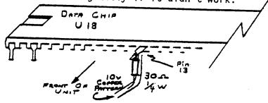
The above drawing shows exactly how I did it, with one word of caution. Don't over heat pin 13 when soldering on the resistor. You may damage the data chip and have to replace it.
